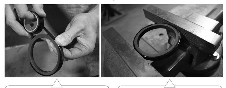
Figure 20 Piston Ring Assembly for Model 391 Valves (Step 1)
