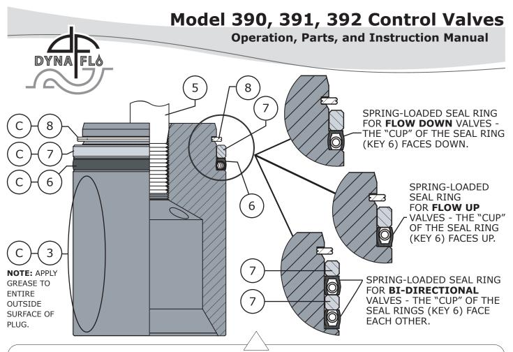
Figure 17 Model 390 Plug Seal Standard Assembly
