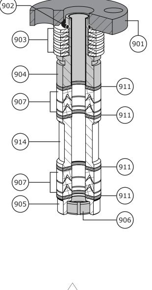
Figure 30 Live Loaded Packing Example
