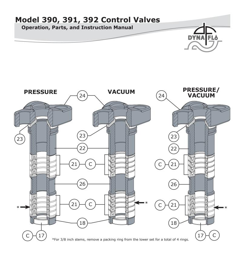
Figure 28 390 Series Control Valve PTFE Packing Diagrams
