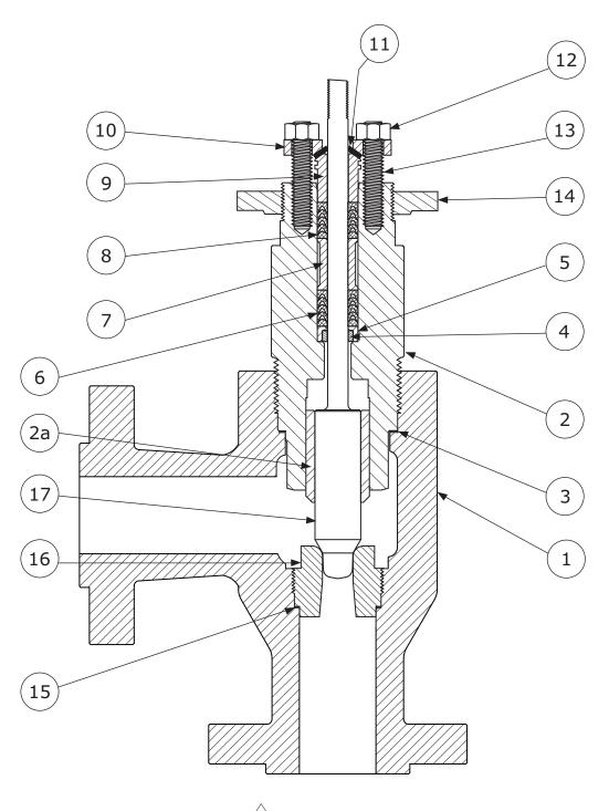
**Figure 5** Typical DF2000 Angle Body Assembly with Flanged Connections
