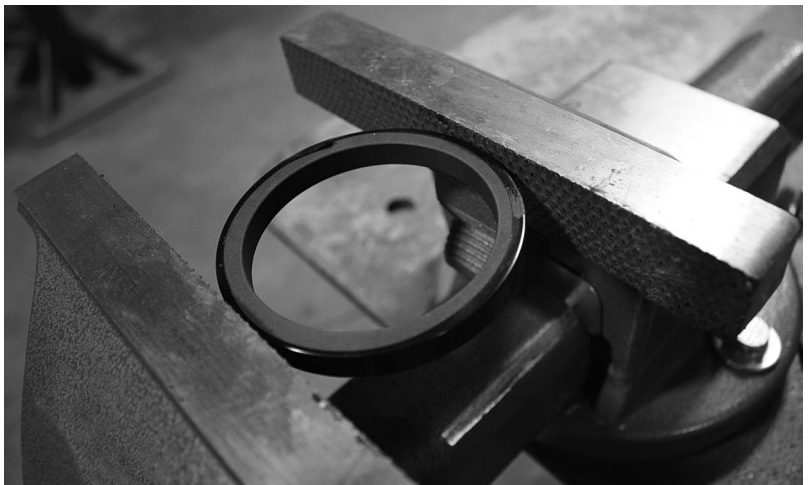
Figure 22 Model 361 Piston Ring Vise Break Method (Step 2)
