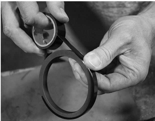
Figure 21 Model 361 Piston Ring Vise Break Method (Step 1)
