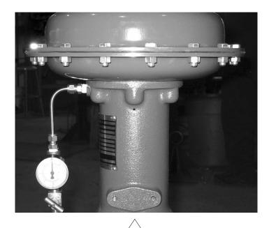
Figure 3 Supply Line and Gauge
