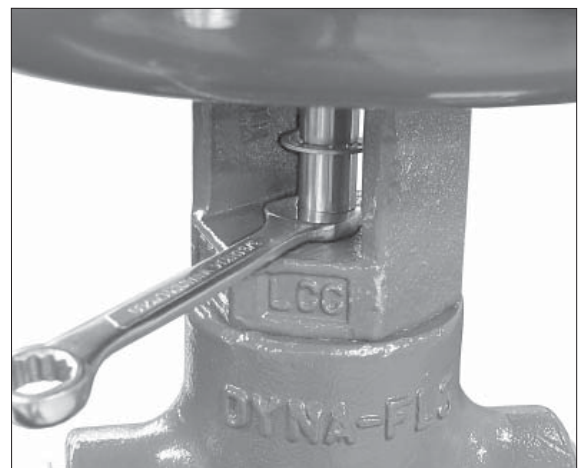
Figure 4 Wrench / Stem Flat Detail
